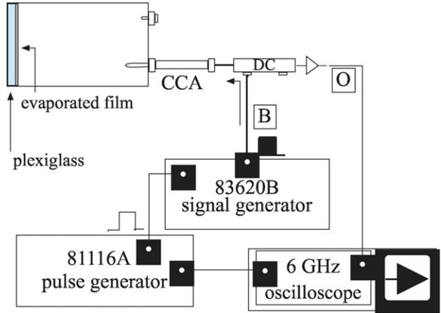
Fig. 2. Experimental setup for the measurement of the parameters of the cavity  $\nu$  and  $Q_{exp}$ .
