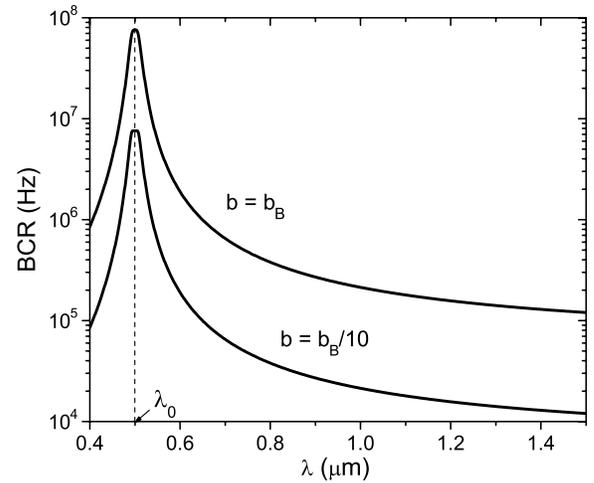
FIG. 2. Bright counting rate as function of wavelength of the field for different values of  $b$ , showing that the BCR increases proportionally to  $b$ . The resonant wavelength is  $\lambda_0=500$  nm.
