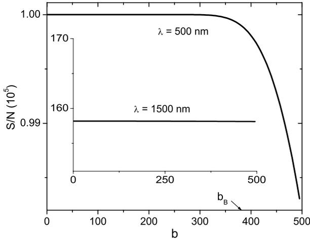
FIG. 1. Signal-to-noise ratio as function of  $b$  at resonance ( $\lambda=500$  nm) and far from it ( $\lambda=1500$  nm) in the inset. The estimated breakdown value is  $b_B \approx 380$ .
