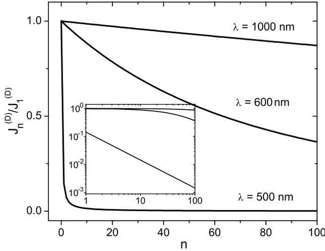
FIG. 4. Normalized dark-count term as a function of  $n$  at breakdown  $b_B$  for different field wavelengths and the same graph in double-logarithmic scale in the inset.
